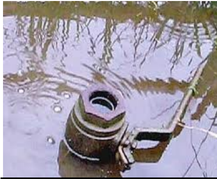
Methane gas escaping from a test well near Whiporie
